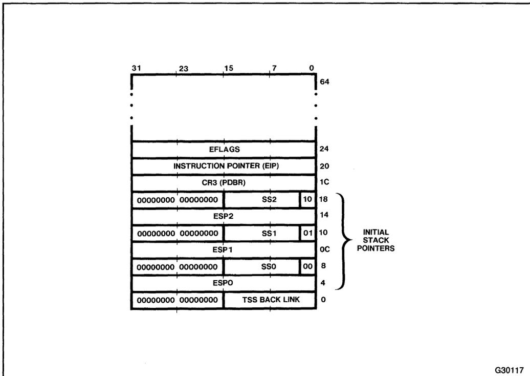
Figure 6-8. Initial Stack Pointers of TSS
