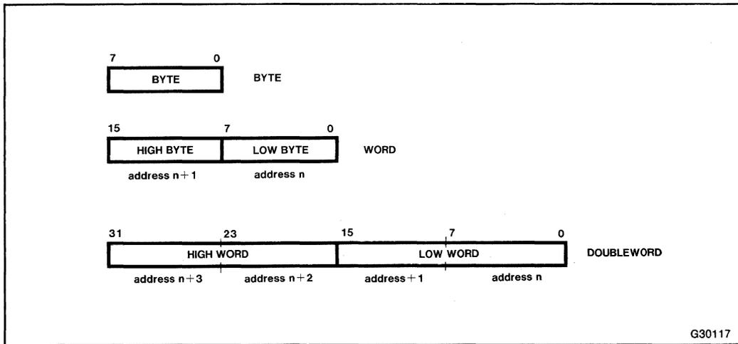
Figure 2-2. Fundamental Data Types
