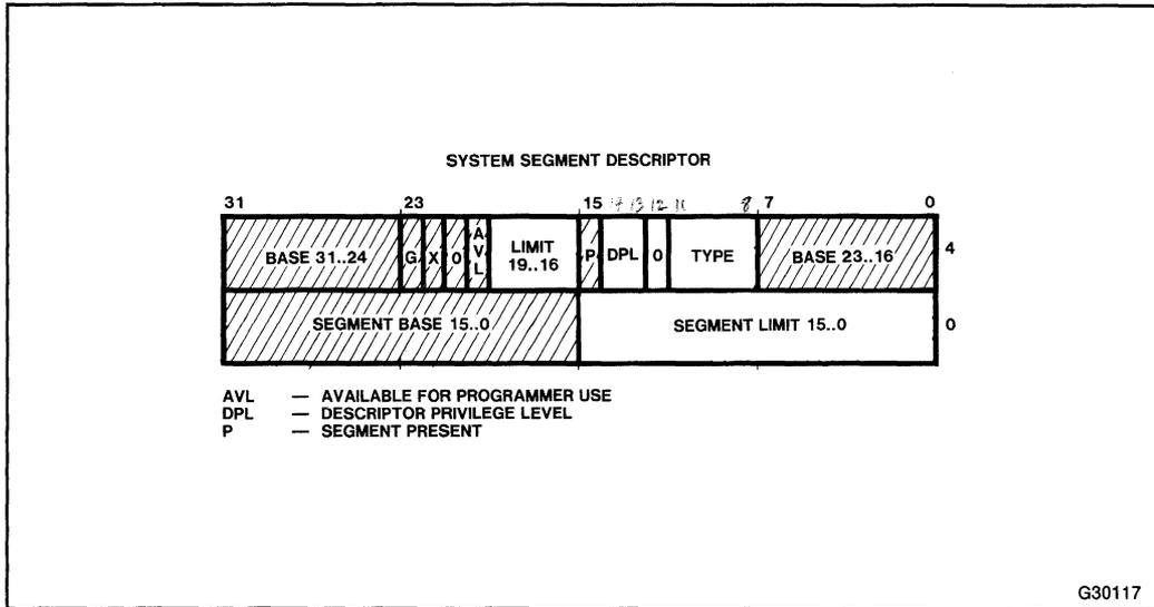
Figure 6-1. Protection Fields of Segment Descriptors (part 2 of 2)
