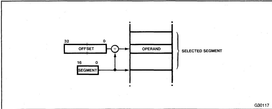
Figure 2-1. Two-Component Pointer
