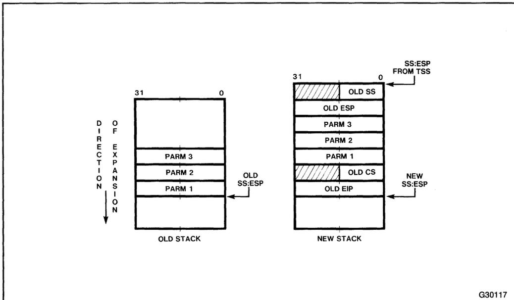
Figure 6-9. Stack Contents after an Interlevel Call
