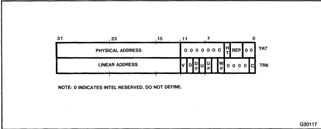
Figure 10-4. Test Registers
