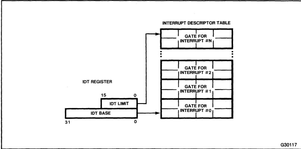
Figure 9-1. IDT Register and Table
