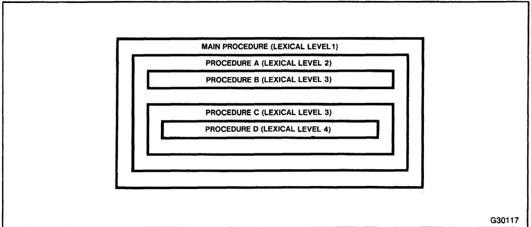
**Figure 3-17. Variable Access in Nested Procedures**
