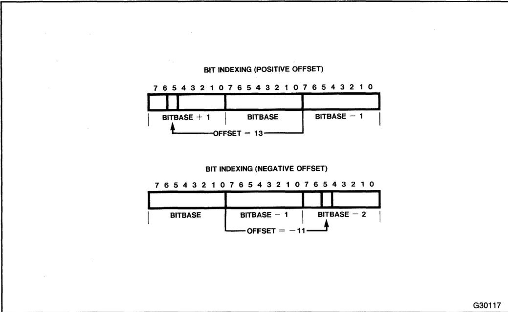
Figure 17-4. Memory Bit Indexing
