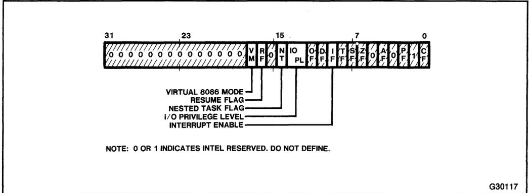
Figure 4-1. Systems Flags of EFLAGS Register
