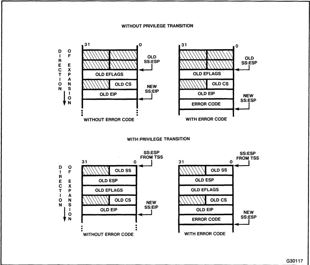
Figure 9-5. Stack Layout after Exception of Interrupt
