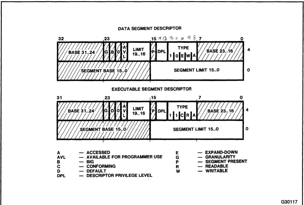
Figure 6-1. Protection Fields of Segment Descriptors (part 1 of 2)
