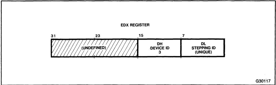
Figure 10-1. Contents of EDX after RESET
