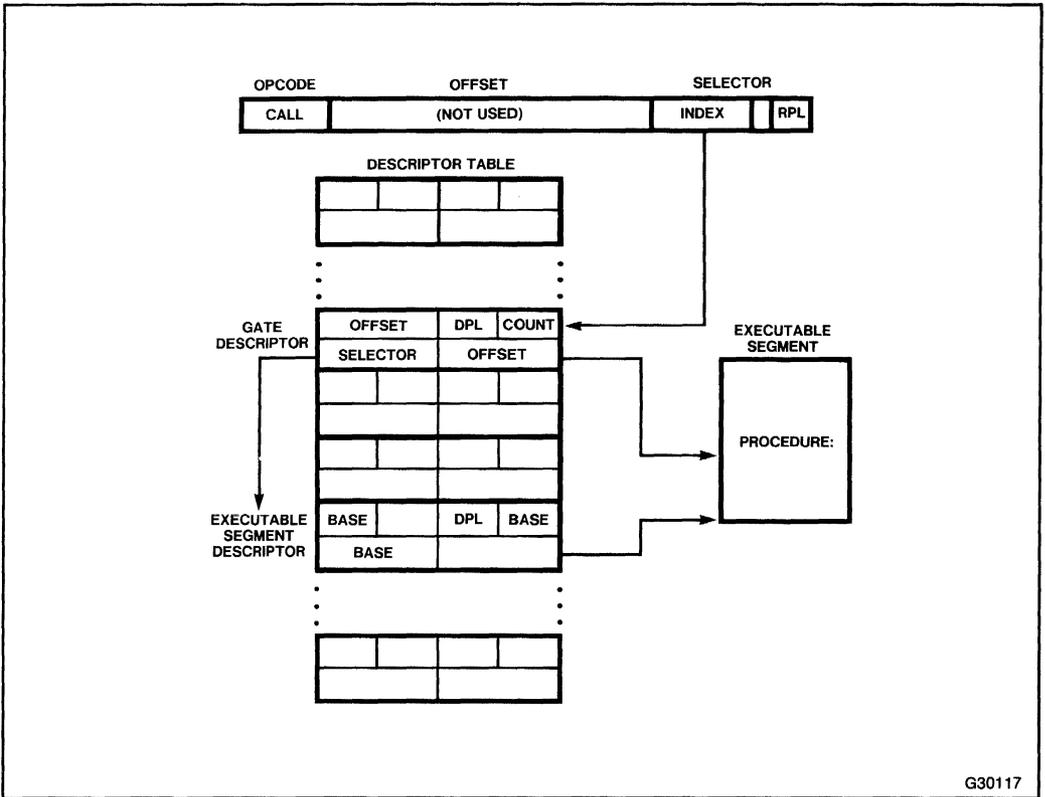
Figure 6-6. Indirect Transfer via Call Gate
